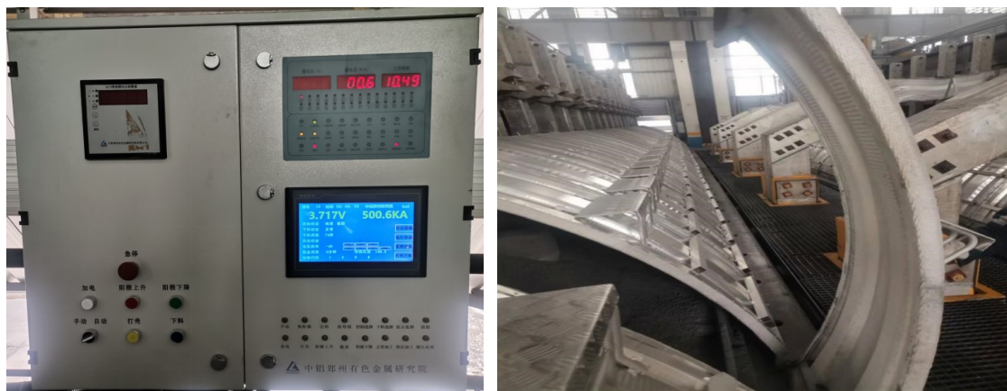
Figure 7. Left: Intelligent control system for FHEST 3.0 technology test cell, Right: Insulated hoods for FHEST 3.0 technology test cell.
